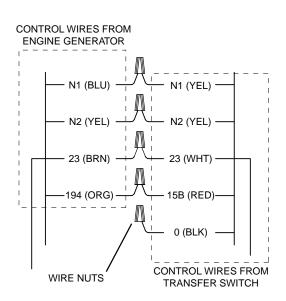
Figure 3. Wire Connections
